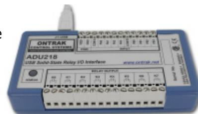
1. Connect the external GPI module to a free USB port of the server system unit. You do not need to install any drivers, once the initialization is complete, the Status LED on the USB module should change from red to green.
