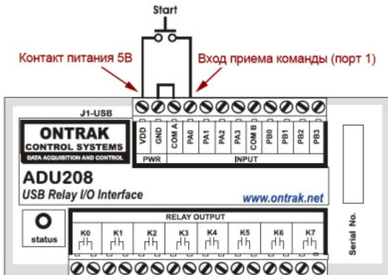
The GPI command receiver is triggered when the TTL level voltage is applied to the corresponding USB module input PA 0...3 or PB 0...3. In order to ensure triggering by a button with so-called “dry contacts”, it is necessary to make connections according to the diagram shown in the figure.
