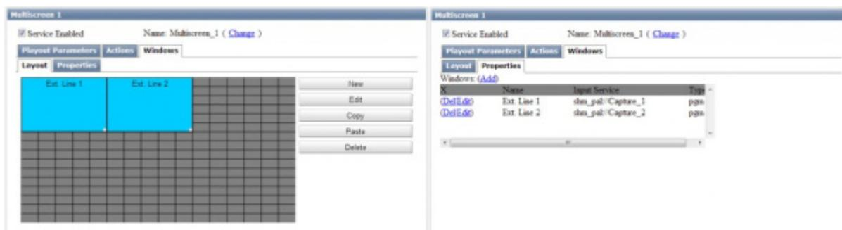
At this point, window editing is complete. As a rule, most of the composition windows contain identical parameters. To copy the windows, you need to use the Copy/Paste buttons in the Windows Layout tab. You can set the size of each window by pulling the white marker at the bottom right of the window.
