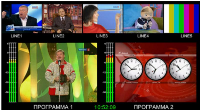
The SL NEO server in any series can be equipped with optional SD/HD SDI and/or HDMI outputs to display all input and output signals on the SDI/HDMI monitor screen in MultiScreen mode.
