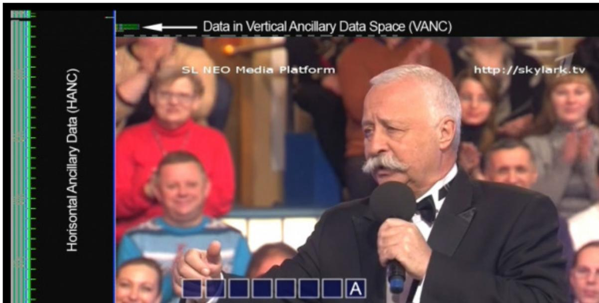
To generate tags in the output SDI signal of the SL NEO server, you must enable VANC-interval data generation (SMPTE 291M standard) with the Use VANC parameter: Administrator Control Panel→Manage→Video IO Boards→Playout\_N→Edit (second from left)→Configure Service→General→Use VANC.
