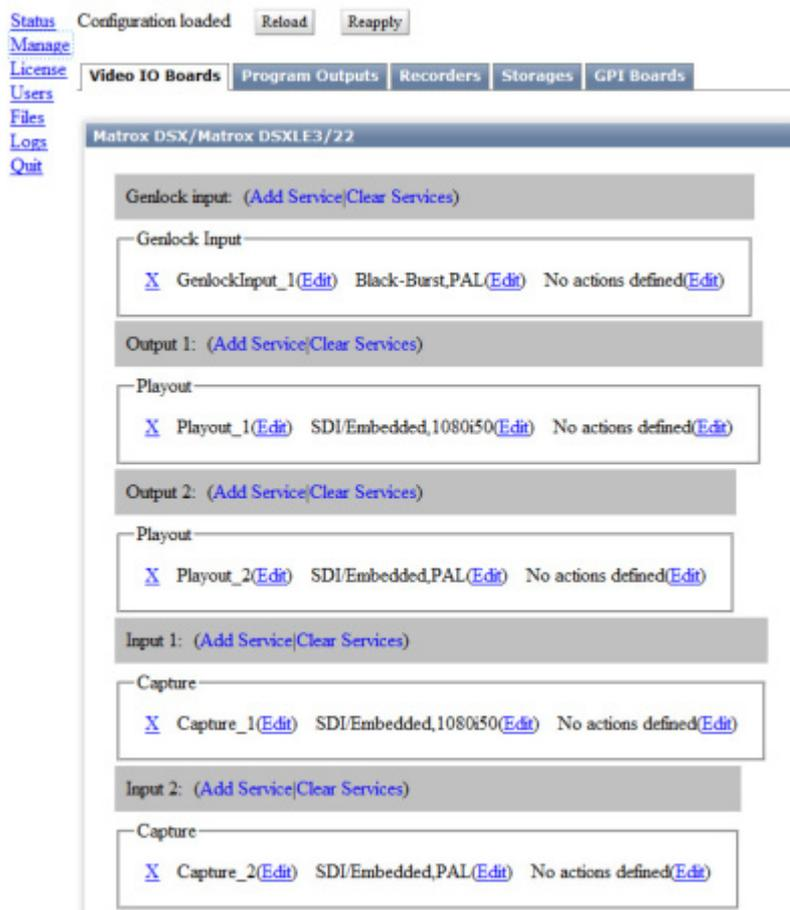
The Genlock window is designed to activate the external synchronization mode of the output devices. You can change the settings by pressing the Edit button next to the current mode (Black-Burst, PAL in
