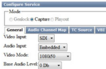
The Input 1 window displays the current settings for the Matrox DSX.LE3/22 board's first input. You can change the settings by clicking the Edit button, next to the current mode. In the Configure Service window you can see and change the capture channel settings.
